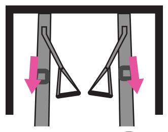
**NOTE:** The rods should be positioned on the opposite side of the door from the swing. You should NOT be able to see them!
